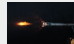
Muzzle flash with an A1 bird cage flash hider, M4 carbine with 14.5" barrel.
