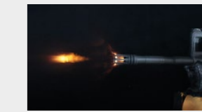
Muzzle flash with an A1 bird cage flash hider, M4 carbine with 14.5" barrel.
