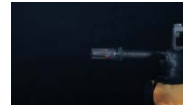
Muzzle flash with an Ase Ultra HiPer flash hider, M4 carbine with 14.5" barrel.
