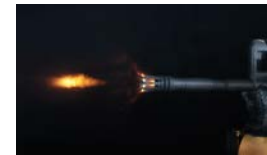
Muzzle flash with an A1 bird cage flash hider, M4 carbine with 14.5" barrel.
